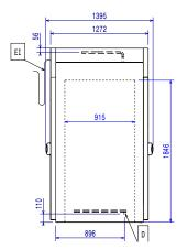
Drain Electrical inlet (power) RO Refrigerant Outlet
